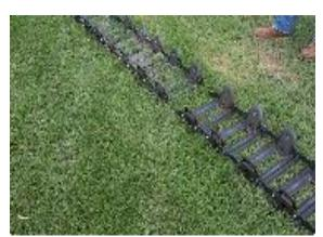
1. Your track is delivered with minimal assembly required. In some cases, your track may be delivered in sections for ease in handling. You may have to pre-assemble two sections to create a track side. Be certain to verify that each side of your pre-assembly has the same number of track pads.
