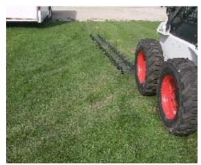
5. Repeat the procedure for the other side. The track sections are now ready to be rolled and stored until they are re-installed. For prolonged storage, it is best to pressure wash, and spray with a light duty oil (WD 40)
