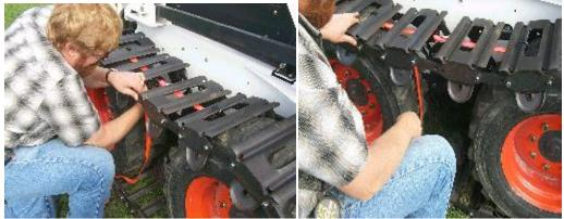
9. Attach the come-along to the underside of the track on both ends through the bottom opening of the second track. This will provide the most even joining of the track sections.
