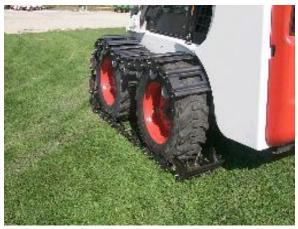
6. Pull the front of the track over the front wheel, taking up as much slack as possible. Check for clearance! Remember - any modifications to the skid steer that are necessary are the responsibility of the owner.
