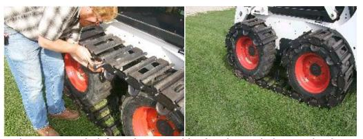
1. Loosen and remove two bolt from the assembly. Let the track drop on the tires.
