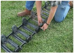
2. Assemble the two components for each side of the track, fastening the links with the bolts provided.
