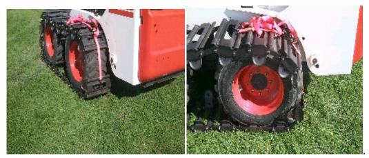
7. Attach a common come-along (obtained at any hardware store) to both ends of the track. Ratchet any slack.
