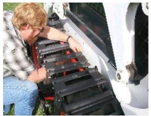
11. Loosen the come-along. Slide the come-along to the far side of the track. Ratchet the comealong until the linkage lines up with the mounting hole. Insert the bolt and hand tighten the locknut.
