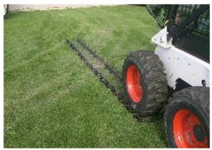
4. Drive the skid steer onto the track.
