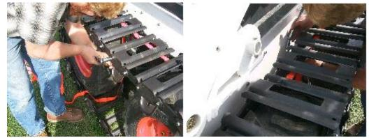
12. Check to make sure there is ½-3 inches of slack in the track. Linkages of one or more track pads can be adjusted to obtain this measurement. When you obtain the desired amount of slack, tighten bolts from the assembly and any adjustment made.
