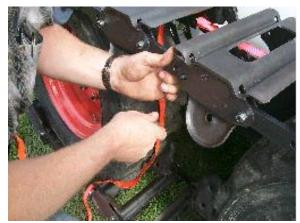
10. Ratchet the come-along until the linkage lines up with the mounting hole of the other track. Insert the bolt and hand tighten the locknut.
