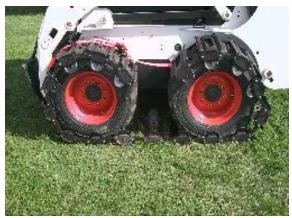
8. Drive the skid steer forward to bring the back of the track to the middle position as shown.
