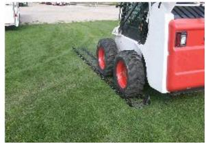
5. Stop when the back wheel of the skid steer passes the first track pad.
