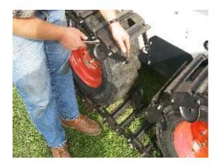
2. Replace the bolts and nuts to the links to prevent misplacing them.
