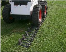
3. Pull the track off the front tire and lay it on the ground.
